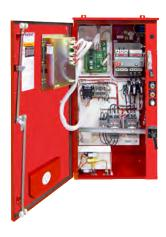
Description—Firetrol\* FTA1300 Wye-Delta, Open Transition Starting Fire Pump Controllers are used with delta-wound squirrel cage motors. FTA1300 controllers are of the open circuit transition type in which the motor circuit is opened during the transition from start to run. The controller monitors, displays and records fire pump system information.
